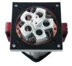
Connection terminals in plugs and sockets 200 A for conductor cross sections of 70 to 150 mm², 250 A and 400 A for conductor cross sections of 70 to 185 mm² or with flexible conductors, and 70 to 240 mm² with single or multiple strand conductors.
