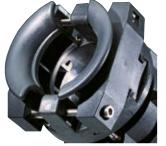
Plugs, connectors, inlets and wall mounted receptacles are supplied with flared bushings for cables of diameter 45 to 65 mm. The outside cable grip facilitates connection.
