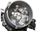
Two pilot contacts are a standard fitting in all plugs and sockets. The pilot contacts lag when the plug is inserted and lead when it is withdrawn. If required, plugs and sockets can be electrically interlocked.
